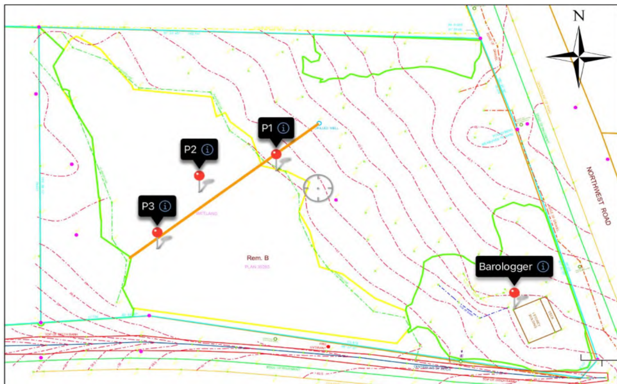
Figure 1. Topographic site plan showing the locations of Piezometer installations and hand augered soil test sites labelled P1-P3 within the subject wetland (yellow outline).
