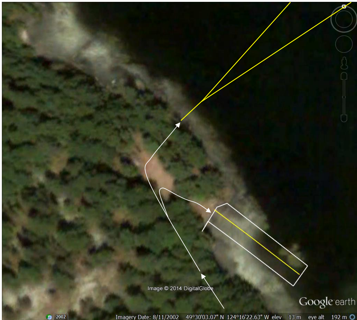
Figure 19. Image from Google Earth showing approximate location of wharf (upper lines, drawn based on McDiarmid survey [BCLS1920]) and lot 280 (float and ramp; lower lines, based on Matthews survey [BCLS1957] and capped pin locations). Tucker Bay Road approaches these two water access locations from the southeast (indicated with an arrow), near the shore, and enters the open area near the approaches to the wharf and float sites.
