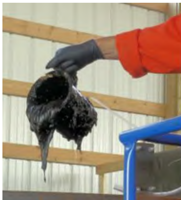
Diluted bitumen after about nine days of weathering at about 15°C. A lower temperature typical of the Salish Sea could increase thickness seen here.
