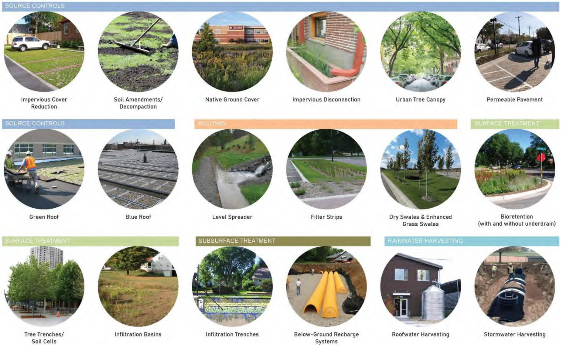
Figure 6: Green Infrastructure Rainwater Management Techniques
