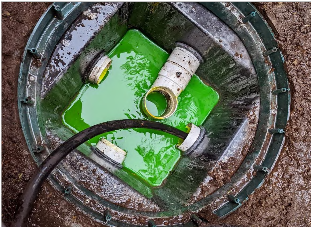
Picture 7: Inside d-box during flow & dye test
