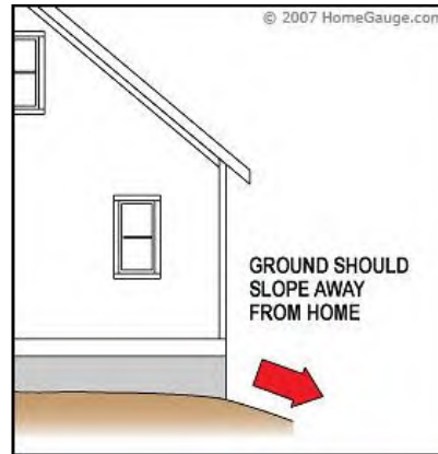
3.3 GROUND SLOPE AT FOUNDATION (Picture 2)
