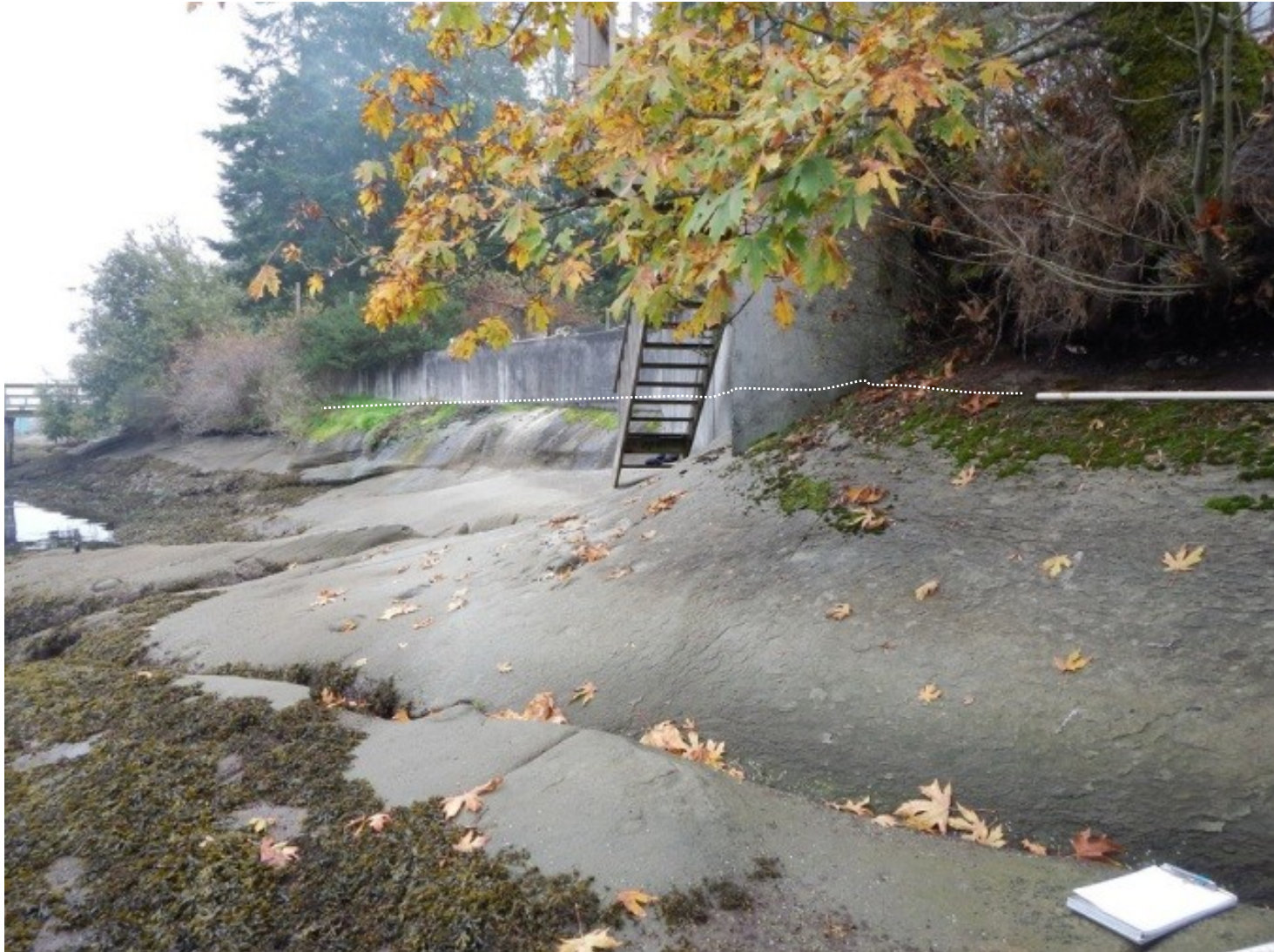
Figure 5. The natural boundary was estimated to be 5.0 m above tidal datum, as measured to the base of the roots on the property just to the west of 260 Cayzer Rd. The dashed line indicates the approximate extension of the elevation across the property.
