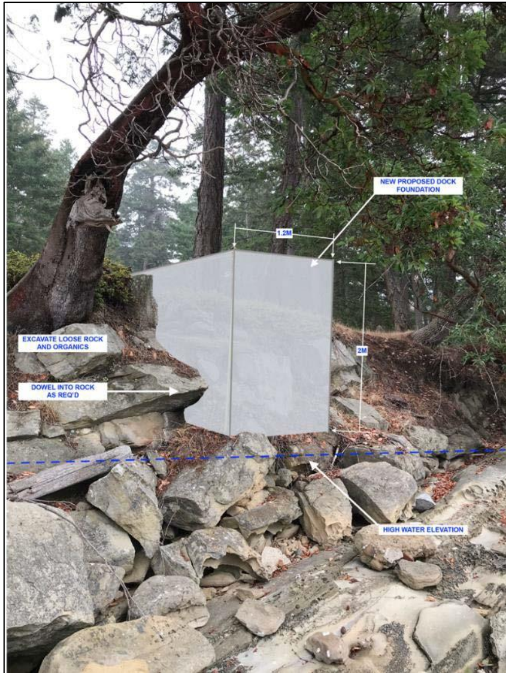
Detail Image of Abutment Structure
