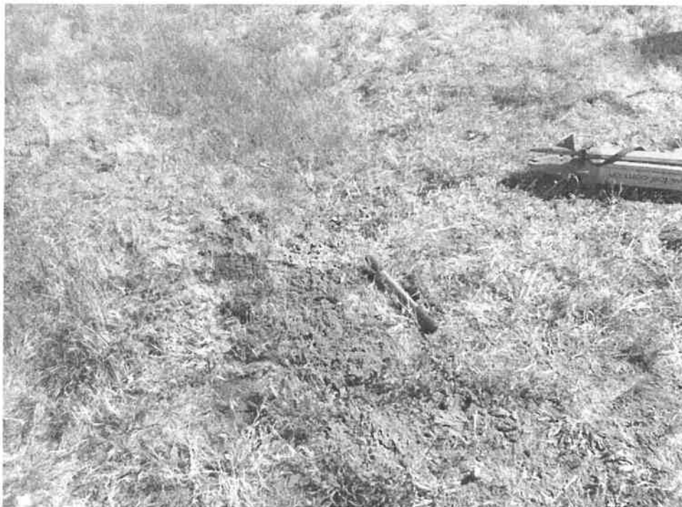
Photograph 4: Hand auger depth of sand deposits within the area of proposed development.
