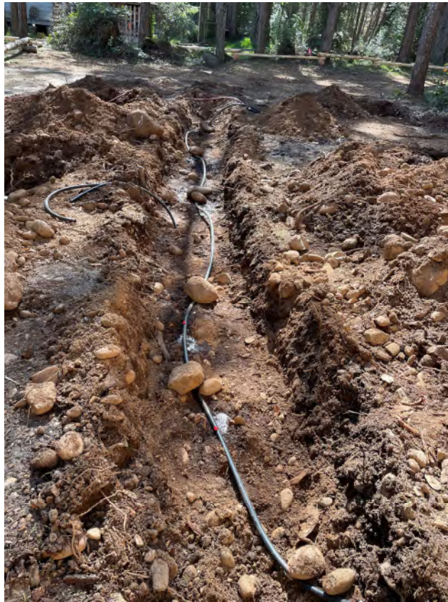
Photo. 3 Test trench dug in area of proposed wastewater dispersal field. The pipe with emitters had been discharging water for over 24 hours at a rate of about 750 Litres per day
