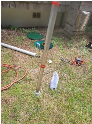
Tank "sludge judge" sample – minimal solids
