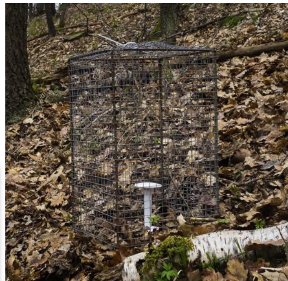
Figure 3. TMS data logger measuring air, surface, and soil temperatures and soil moisture, protected by wire cage from herbivorous animals. Reproduced from Wild et al. 2019 2 Figure 1 (Left) and Figure 8 (Right).
