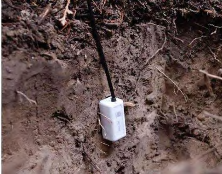
Figure 3. Typical soil moisture sensor installation in a shallow (<50 cm), narrow (~15 cm wide) hole.
