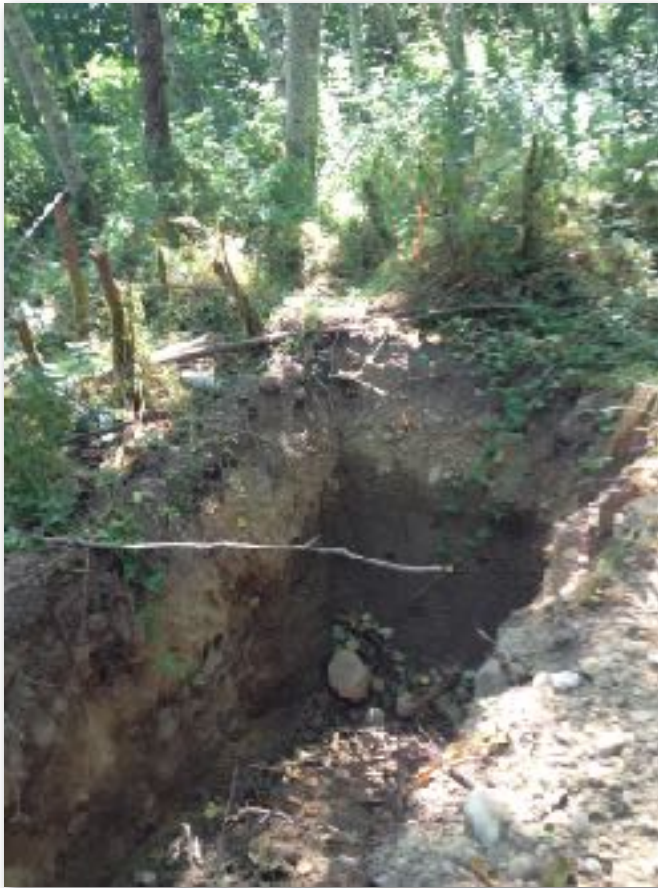
Figure 7. Percolation test northeast of the pond in septic field showing young alder forest, topsoil and colluvial deposits.
