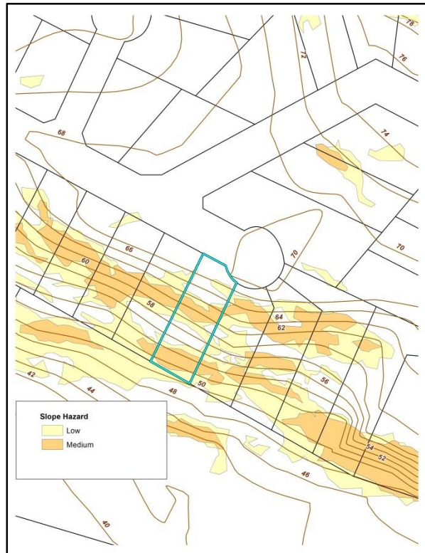
Figure Three: Slope Hazard and Contours
