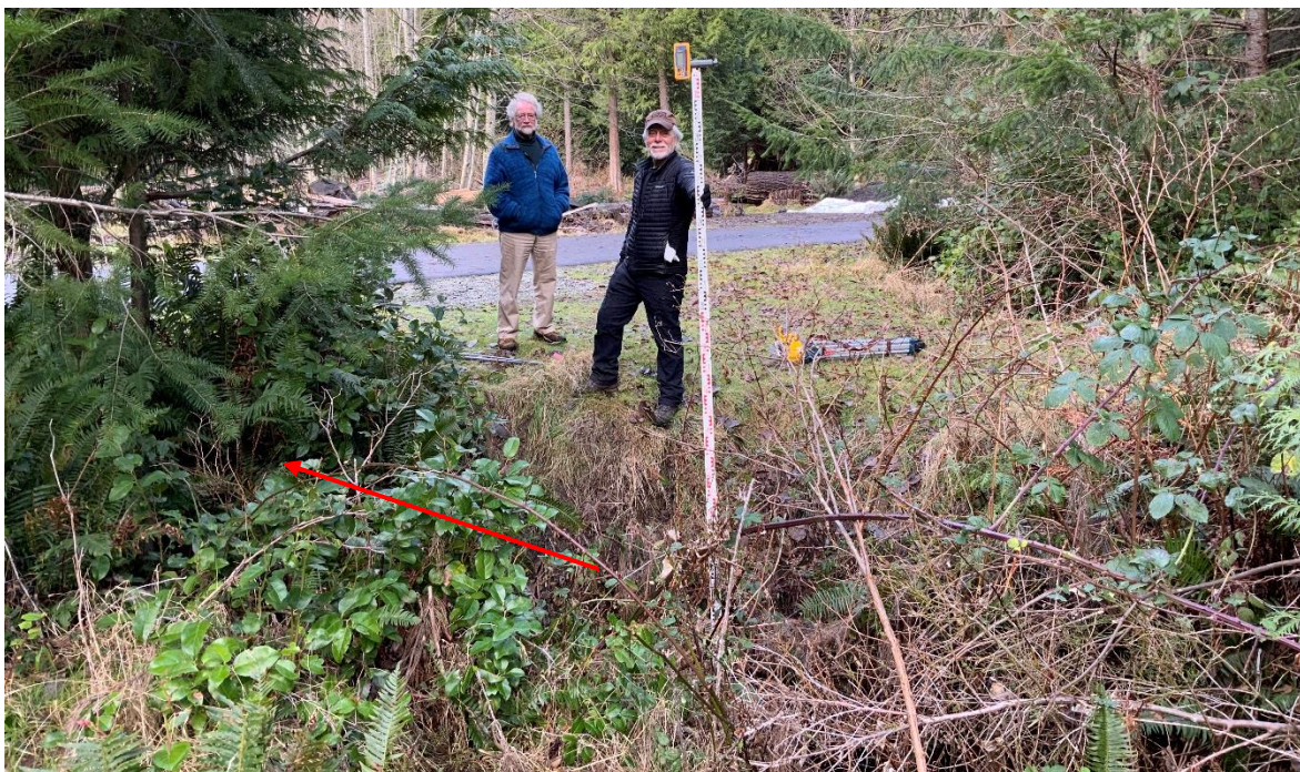
Figure 5. David Brown measures a ditch that is 1.5 metres deep and over 2 metres wide on the east side of the existing driveway on proposed Lot 1. The red arrow shows the direction of water flow in the ditch.
