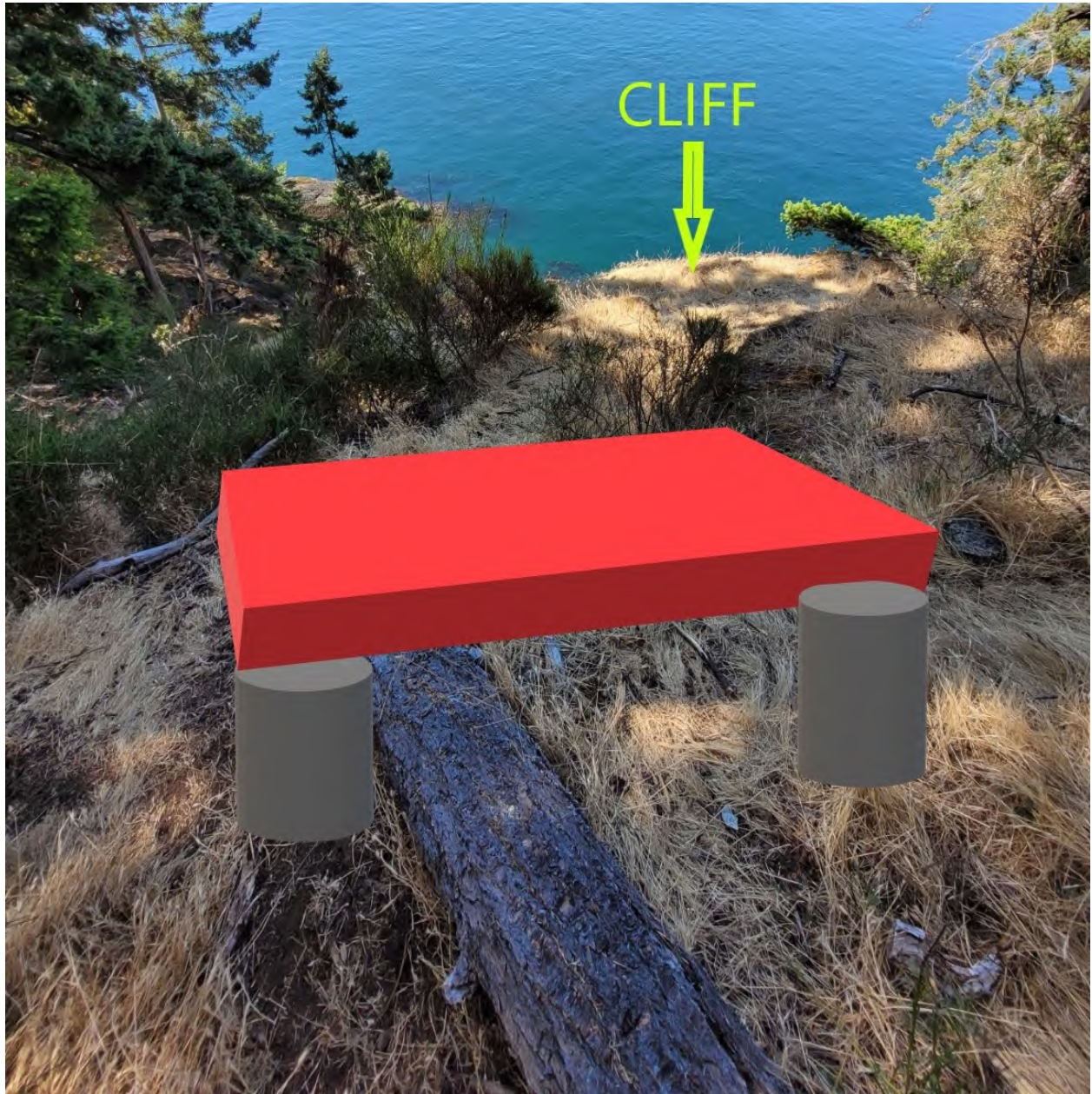
Figure 5: Mockup of final landing of staircase.
