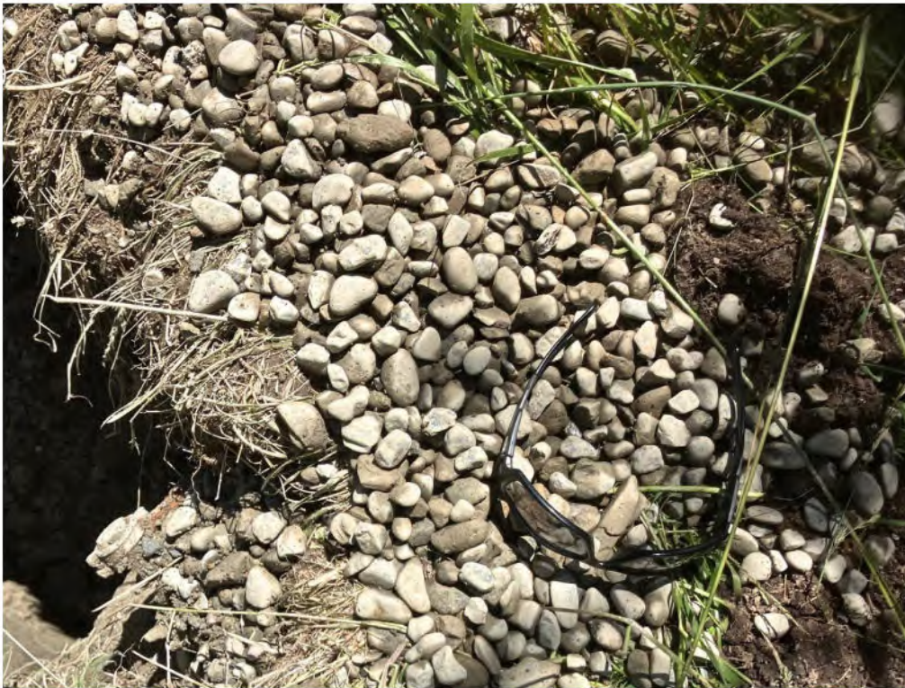
Photo 6. Gravel with sand material for backfill around slotted section of well casing, June 30, 2025.
