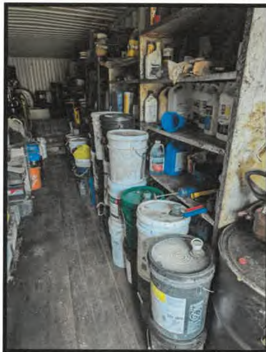
Photo 12: Mechanical fluids storage in sea can with welded lip and secondary containment at rear for spent fluids.
