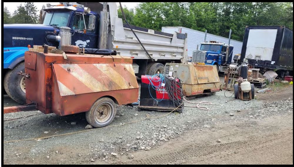
Photo 15 – Air compressors requiring drip trays.
