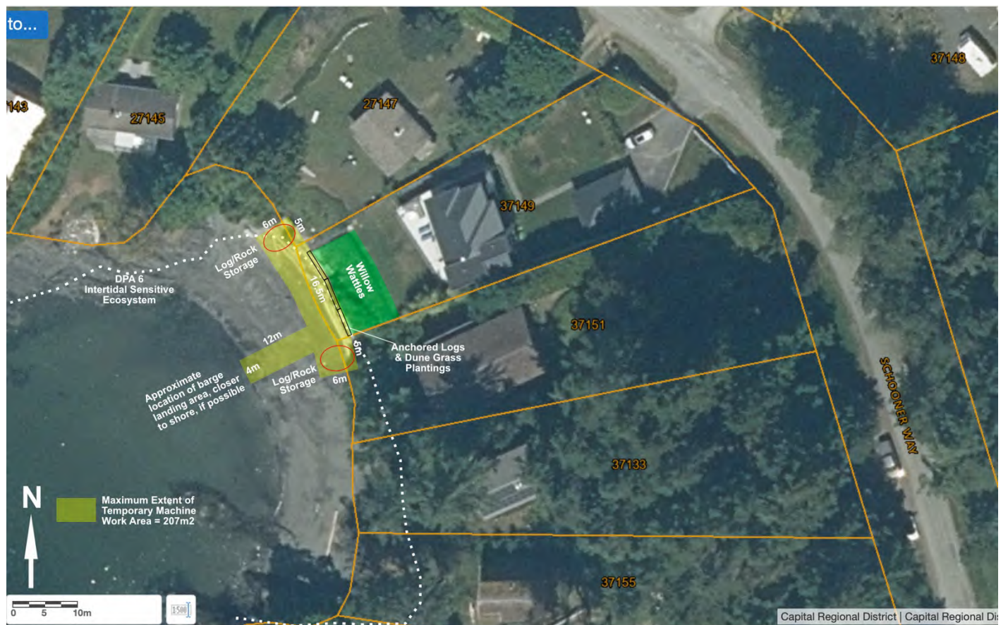
Figure 3. Proposed Green Shores/Bioengineering stabilization work on the shoreline slope at 37149 Schooner Way, and proposed work in DPA #6 – Intertidal Sensitive Ecosystem from OCP Schedule N: anchored logs, willow wattles, and dune grass plantings; and temporary access and temporary disturbance area for small barge, heavy equipment and materials.
