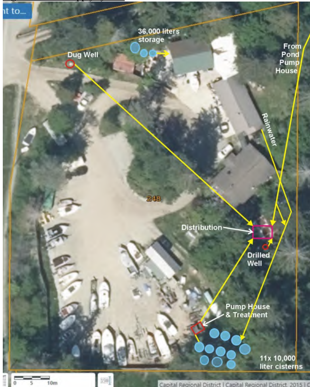
Figure 2: Water supply system
