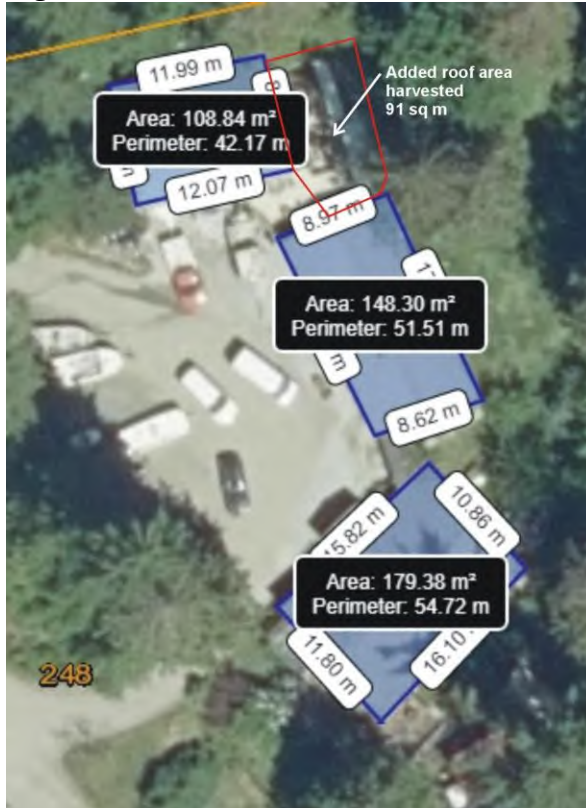
Figure 5: Available roof area
