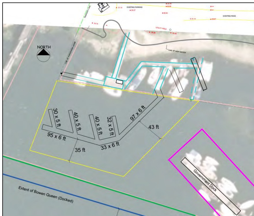
Figure 3: Proposed expanded marina dock configuration
