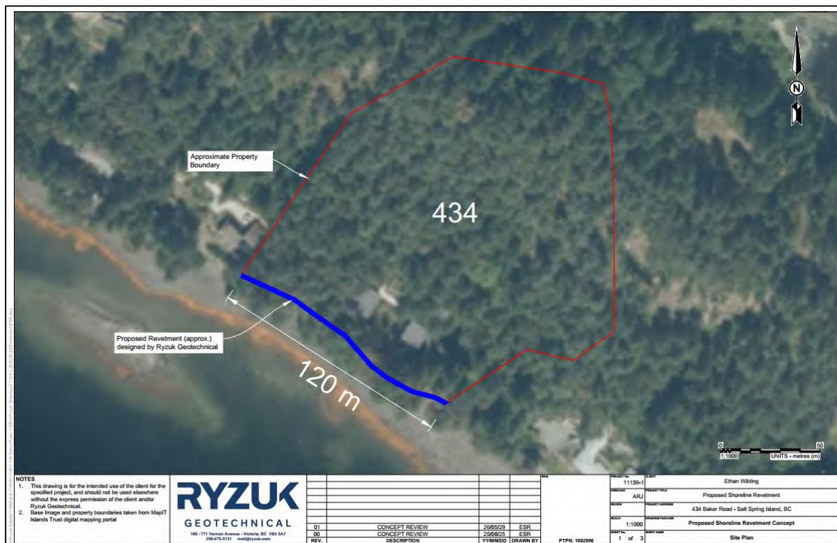
Figure 2: Proposed shoreline revetment location
